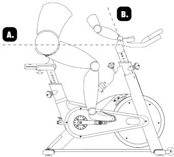
If your ICG IC2 is equipped with a regular 2 way handlebar. If the handlebar is too close to the saddle, your breathing may feel restricted; if the handlebar is too far from the saddle, you may experience back discomfort. To adjust the horizontal position to the handlebar, first dismount the ICG IC2.
