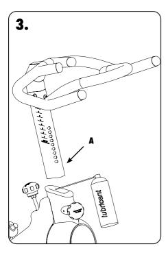
**3.** To maintain the easy adjustability of the handlebar post, the handlebar post should be cleaned and lubricated. First, turn the front adjustment knob counter clockwise and slide the handlebar post out of the frame. Apply a small amount of lubricant spray to a lint-free cloth, and clean the handlebar post **(A)**. Next, apply a small amount of lubricant spray inside of the front frame sleeve.
